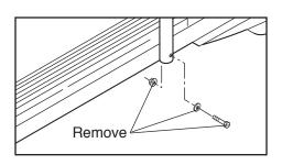
Remove the bolt from the upper end of each handrail.
